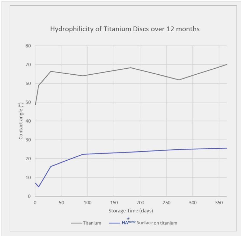
**Figure 1.** HA<sup>nano</sup> Surface modified titanium surfaces are significantly more hydrophilic than unmodified titanium. Results are expected to improve even more with optimized storage conditions.
