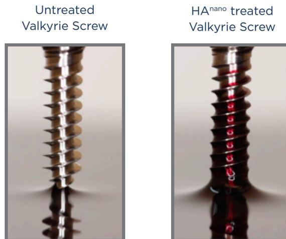
**Figure 2.** The degree of hydrophillticy is greatly enhanced with the HA<sup>nano</sup> surface comaped to an unmodified titanium surface, allowing for facilitated absorption of body fluids into small pores and cavities on the implant surface.
